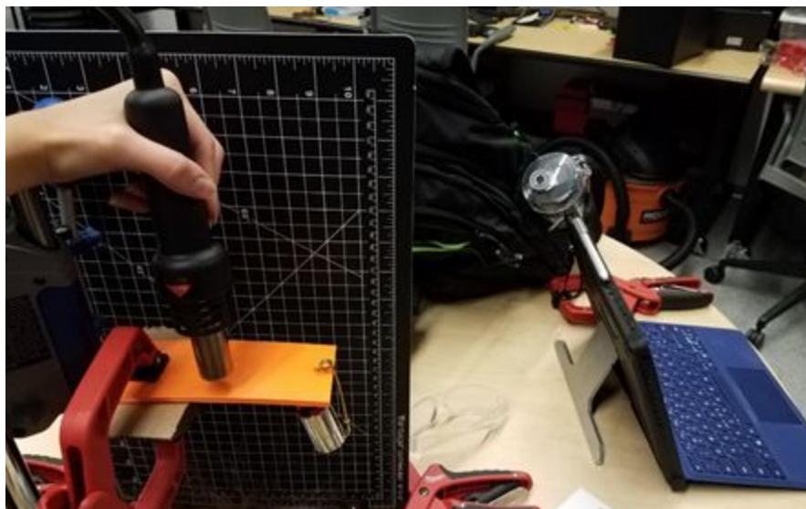
Figure 5.2.3: Visual of How the Heat Was Applied
